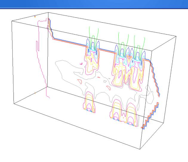
The contour plot is used to display lines of constant temperature on a planar slice through a simulation of a gas-burning furnace.
