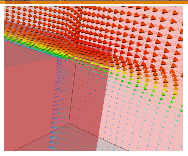
The vector plot close up showing the turbulant flow directly behind the box.
