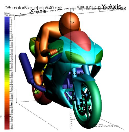
The **subset plot** is used to display different parts of an assembly. Portions of the assembly can be selectively turned on and off..
